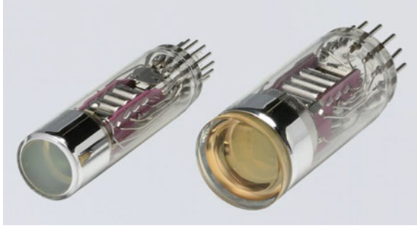
Fig. 6.11 PMTs manufactured by Hamamatsu
